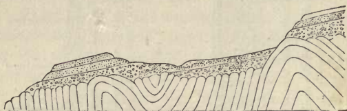
FIG. 8.—Unconformable superposition of Devonian conglomerate on Silurian slates, at St. Abb's Head, Berwickshire.—After Lyell.
